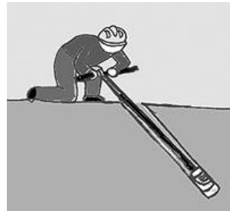
Figure 6. Thread a rod through the eyehole and turn the rod until the anchor expands tightly against the sides of the hole.
