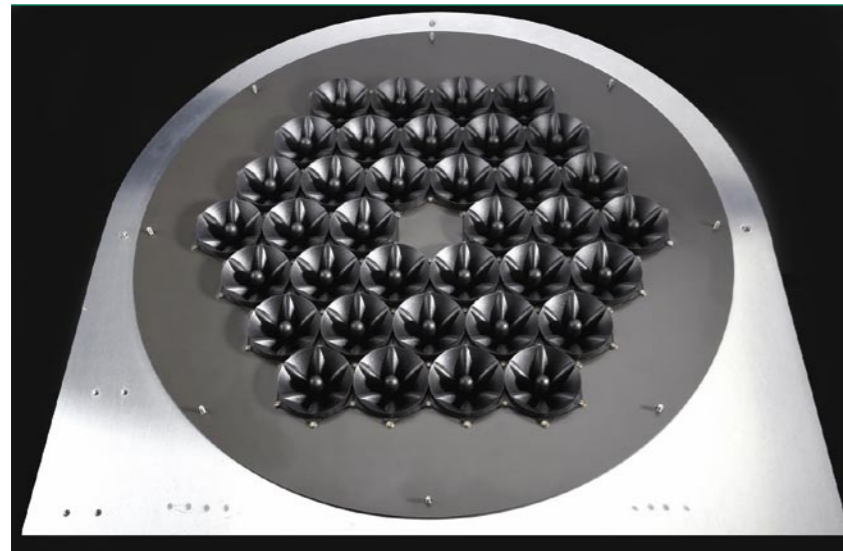
Figure 3. The Triton profiler's six-sided array (patent pending) allows transducers to be spaced more closely than rectangular sodar arrays, producing a more tightly focused sonic beam
