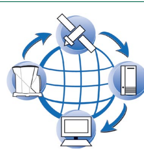
Figure 6. The SkyServe satellite wind data service supplies Triton data every 10 minutes to a secure Second Wind server via the Globalstar satellite network. Users can download the data directly into their analysis systems over the Internet
