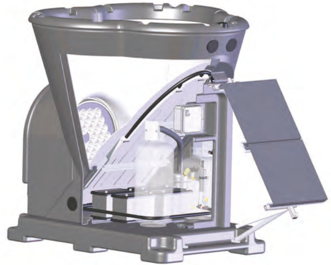
CUTAWAY VIEW OF TRITON WITH MIRROR HEATER SYSTEM. PROPANE CYLINDERS ARE SUPPLIED BY CUSTOMER, AND ARE SHOWN AS TRANSPARENT.
