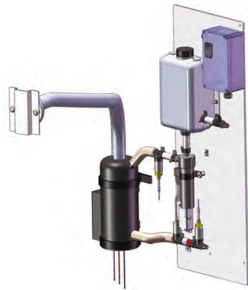
DETAIL SHOWING HEATER AND PUMP ASSEMBLY
